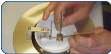
Using the optional PP7465 Advance Sample Handling option allows transfer of pre-frozen specimens
